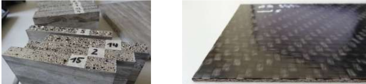
Figure 1. Closed-Pore Aluminum Foam Structure (left), Continuous Carbon Fiber Reinforced Plastic Sheet (right)
